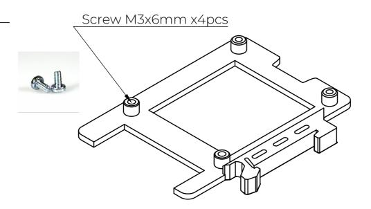
Packaging Contents: 1x DIN Mount plate | 4x M3x6mm screws
