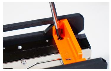
Screw in an HDD Screw (Part 5) into both the FRONT and REAR HDD screw holes
