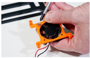
Flip the fan and Fan HAT over and position a fan nut over the bolt and attach the nut to the protruding bolt
