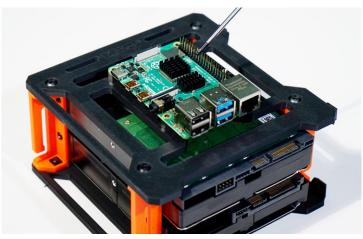
Affix the heat sinks on the RPi BEFORE attaching the Fan HAT (Part 10)
