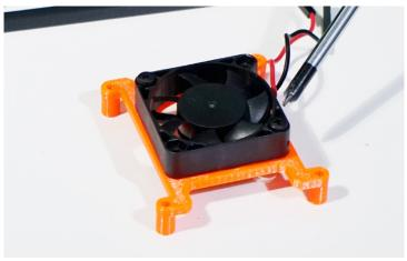
Place one of the bolts from the small plastic bag containing the fan into one corner of the fan and through the Fan HAT
