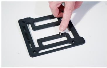
Flip over the RIGHT side plate and screw an M2.5 x 6mm standoff / spacer (Part 8) through the side plate into the M2.5 nut on the other side
