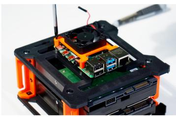
Place the Fan HAT and fan assembly over the RPi.
