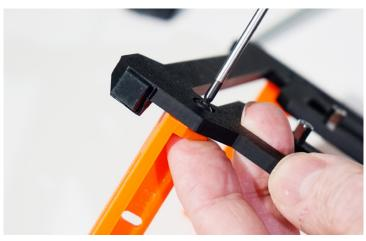
While holding the Square Nut and B Clip in place, loosely tighten the M4 bolt into the Square Nut
