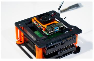
Insert and tighten all M2.5x16 screws to secure the Fan HAT assembly and the RPi to the TPXDuo
