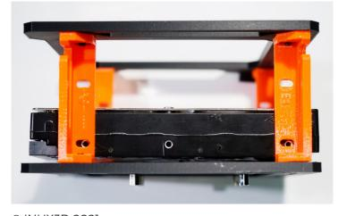
Slide the first HDD so that the holes for the HDD Screws (Part 5) line up between the HDD and the TPXDuo frame
