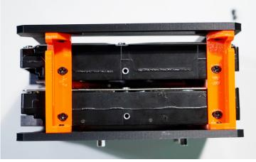
Loosely tighten the remaining 2 screws and you should have an assembly that looks like this from the TOP
