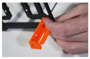
Loosely tighten the bolt into the Square Nut.
