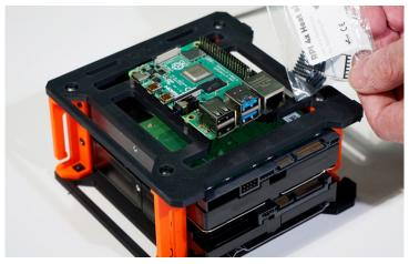
Roughly position the RPi as pictured and prepare to affix the supplied heat sinks to the RPi
