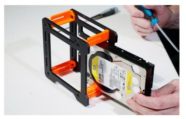
\*The INUX3D logo designates the REAR of the construction Insert one of your 3.5" HDD's from the FRONT of the TPXDUO with the HDD ports also facing the FRONT
