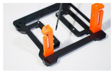
Position a B Clip (Part 4) in the TOP REAR corner of the side plate
