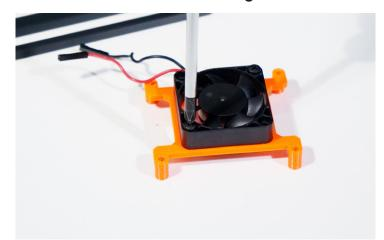
Flip the assembly over and tighten the bolt and nut
