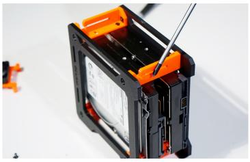
Now insert the second HDD, align the screw holes between the A / B Clips and the HDD
