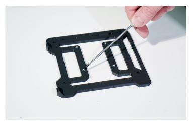
Locate the M2.5 nut recesses on the INSIDE of the RIGHT side plate (Part 1)
