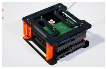
To install your Raspberry Pi, lay the assembly on the LEFT side so that the metal standoffs are facing upward and the HDD connections are facing you
