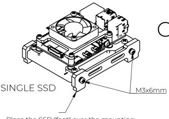
Place the SSD "feet" over the mounting holes and secure them using the M3x6mm screws. Repeat for both sides.
