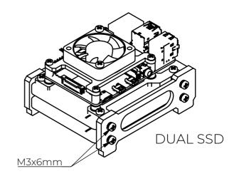
For the Dual SSD version, please mount the SSD "feet" on the TOP SSD drive first and then insert the BOTTOM SSD and secure it as shown, using the M3x6mm screws.
