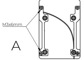
Place the SSD flat on a surface. Place the SSD mounting clips over the holes on the drive and using the M3x6mm screws, secure them.
