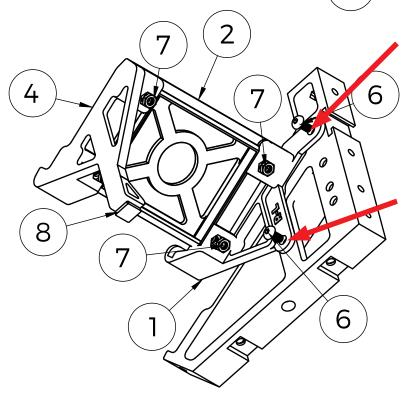
Position the StreamDeck Stand so that its TOP hole lines up with the TOP hole of the PK1 Stand side and push an M4 bolt (Part 6) through. This next bit is quite fiddly, but using your index finger (or tweezers), thread an M4 nut (Part 7) onto the M4 bolt protruding through the PK1 Stand side and tighten the bolt
