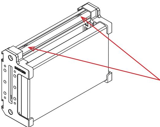
Position the YP cage as shown and note the 2x M5 slide in nuts you dropped in earlier
