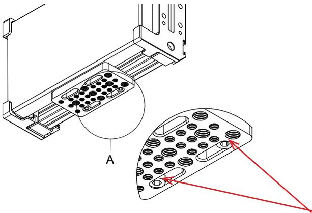
Using 2x M5x8mm bolts, we will **lightly attach** the cheesebar to the slide in T-nuts
