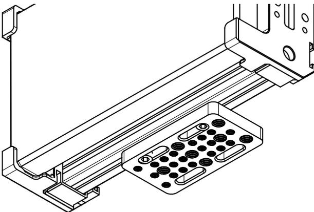
In the event you place your YoloBox Pro such that the HDMI cables are pointing downwards, position the cheesebar so it only covers the aluminium bar and not the YoloBox Pro.
