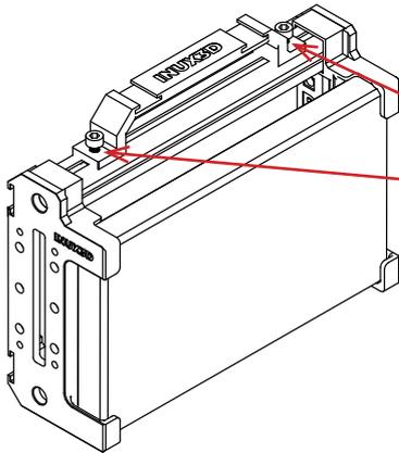
Place the handle on top of the YP cage and **very loosely tighten** the 2x M5x10 bolts into the T-nuts
