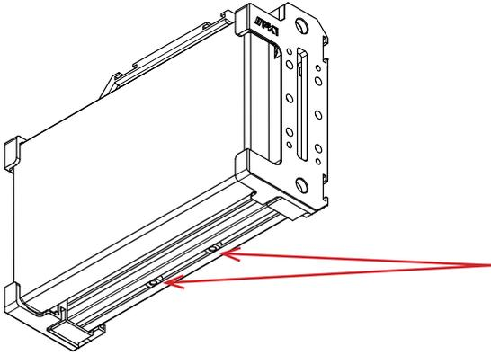
Attaching the cheesebar is like the handle and utilises the two slide in nuts we inserted earlier
