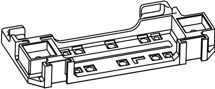
Begin by placing the left side of the YP Cage smooth side down with the cold shoes facing you
