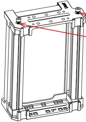
Place the right side of the YP cage over the top of the YoloBox Pro and the 2 aluminium bars
