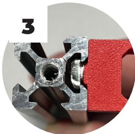
Attaching the cable managers requires the use of an M4x8mm bolt through the cable manager and into an M4 drop in nut.
