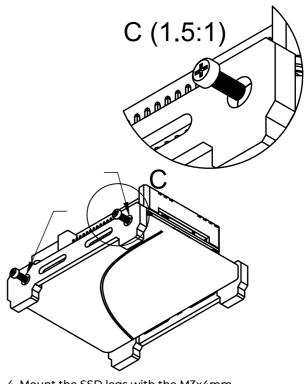
4. Mount the SSD legs with the M3x4mm screws as shown below in Flg. C
