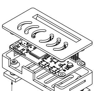
First place the Pi inside the base and align the moutning holes
